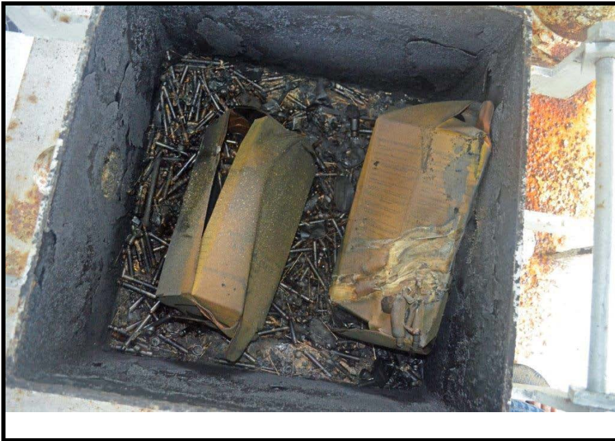
Photo 11: Unburnt solids and sharps in the remnant ash material at Pohnpei State Hospital (taken 07/04/2014 by Natalie Stella ref: DSC0345)
