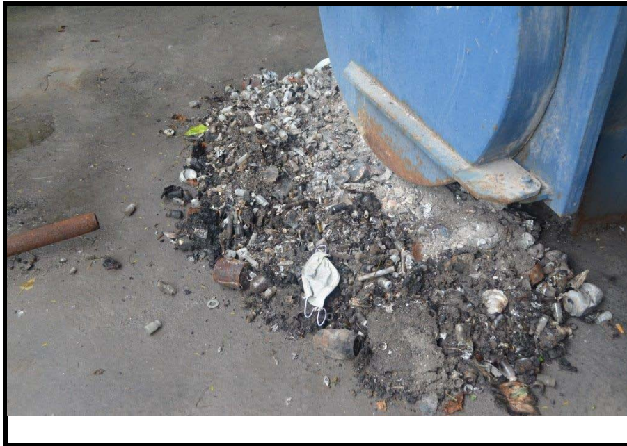
Photo 5: Solids and unburnt sharps in ash material from the Chuuk incinerator (taken 4/04/2014 by Natalie Stella ref:DSC03909)
