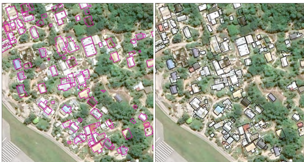
Figure C-1: Example of original building outlines (left) and updated building outlines (right). [Source: SPC].
