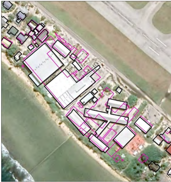
Figure C-2: Example comparison of original (pink) and updated (black) building outlines at the police station. [Data source: SPC].
