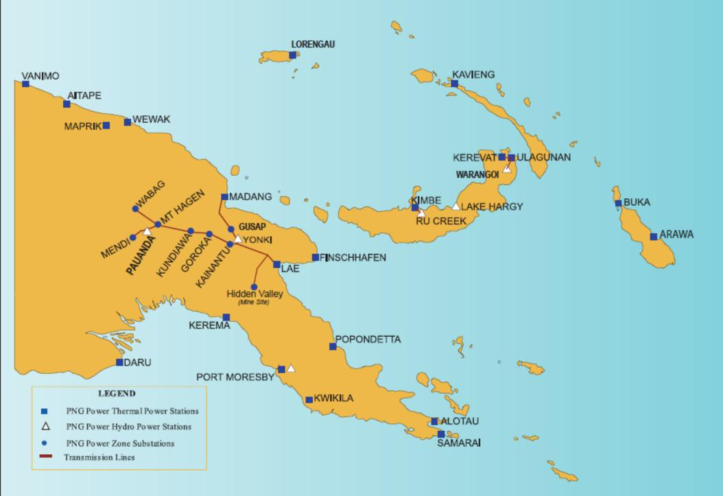
stations account for 70% and thermal account for 30% of the total capacity. The transmission voltages are 132kV, 66kV and 33kV, while the distribution voltages are 11kV and 22 kV. The standard consumption voltages are 415 Volts and 240 Volts at 50 Hz.
