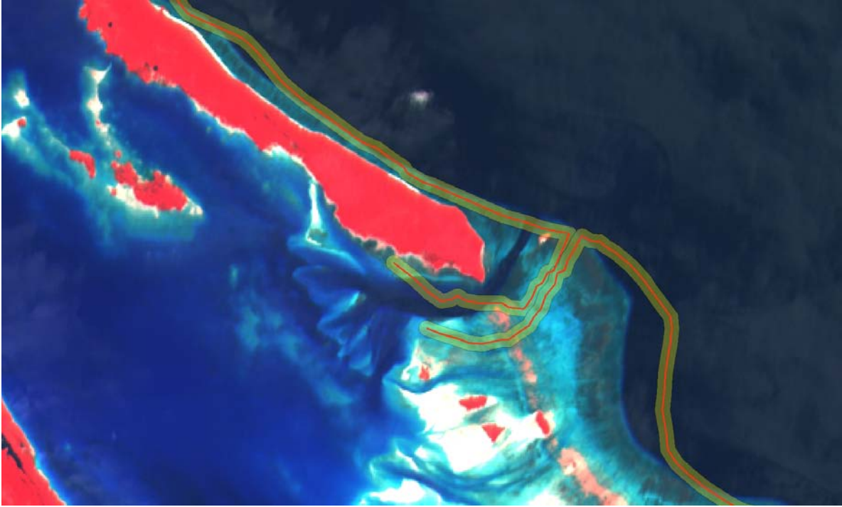
Figure 14: Overlay of the buffered habitat areas on the corresponding SPOT-2 satellite image, showing a shift due to the low geolocation accuracy of the SPOT image
