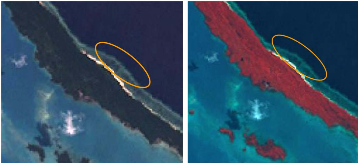
Figure 23: When loading these images into a software like ESRI ArcGIS, particular care should be taken to apply the correct colour stretching, as the colour automatically applied by the software generally gives very light colours, which are not the best for photo interpretation. In ESRI ArcGIS we generally applied a 4–5 standard deviation, which gives a darker and well contrasted image. The black background values (Red=0, Green=0, Blue=0) must be set to transparent.
