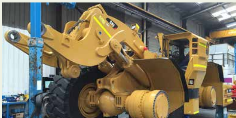
Changing the axles on the Cadia underground loader fleet has improved safety and costs.
