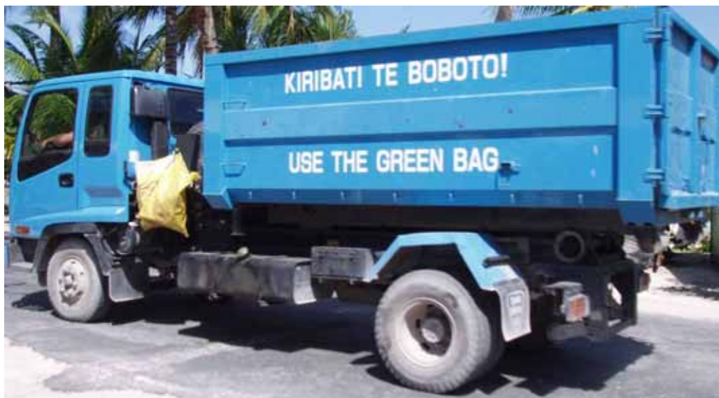
Figure 1: TUC Greenbag roll-on/roll-off collection truck
