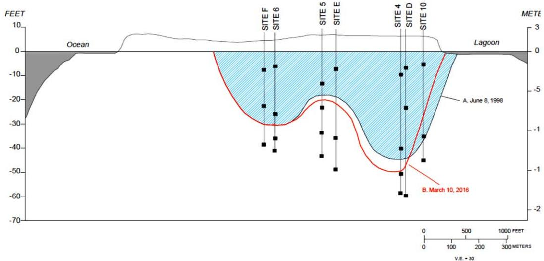
**FIGURE 42.** Diagram of Laura lens monitoring site Number Five. Note the shifting of the water lens in 2016 compared to how it was in 1998 (EPA, 2015).
