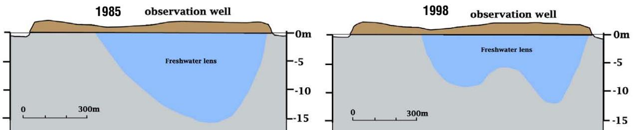
**FIGURE 40.** Diagram of Laura groundwater lens comparison of well Number Five at cross section C between 1985 and the El Nino in 1998 (JIRCA, 2014).
