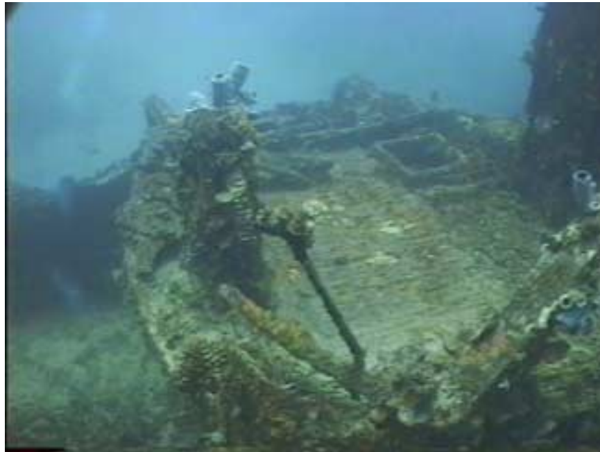
Photo KS4-4 Pilothouse area of North Loi wreck. Notice wood flooring is still intact, and drive gear for ships steering forward of the missing wheel position.
