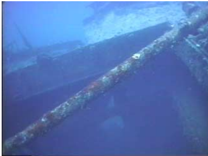
Photo KS10-10 Number 4 hold with damage through hull and at deck level. This damage is what sunk the vessel.
