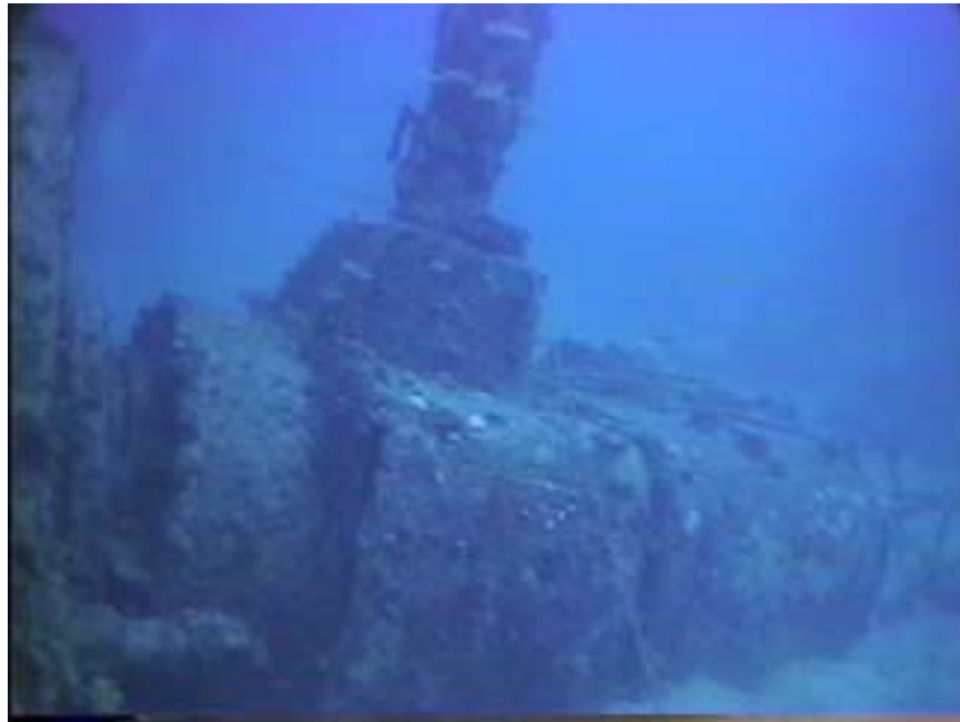
Photo KS13-9 The rear of the fighting bridge at approximately 80 feet. It was crushed over flat against the bottom by the capsizing of the vessel. A large coral mountain rises up to the right of the photo, and a lost anchor and line are visible in the photo.
