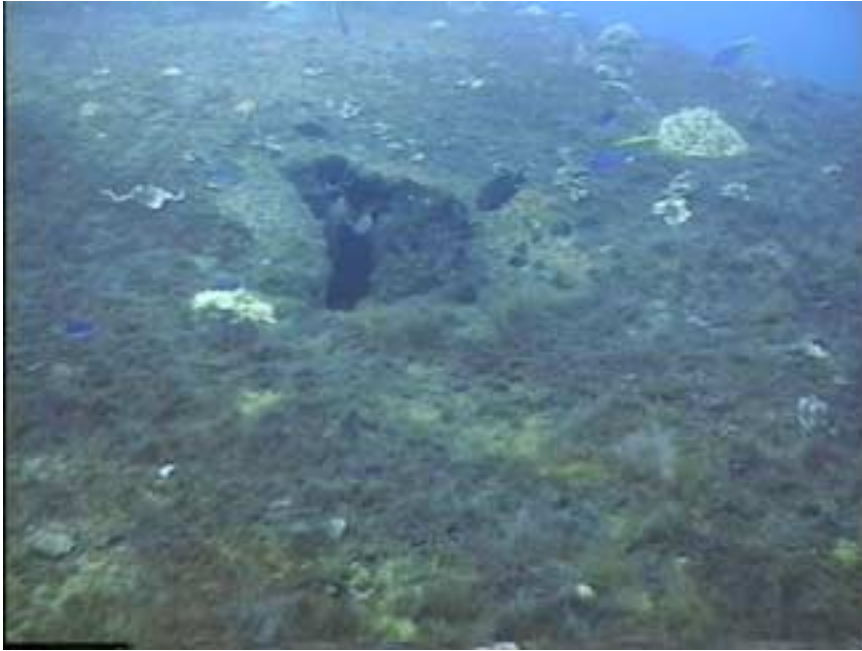
Photo WT12-12. Bomb damage or artillery round hole in the starboard side, just forward of or just in the engine room spaces. Hole measured apx. 3 square feet of area.
