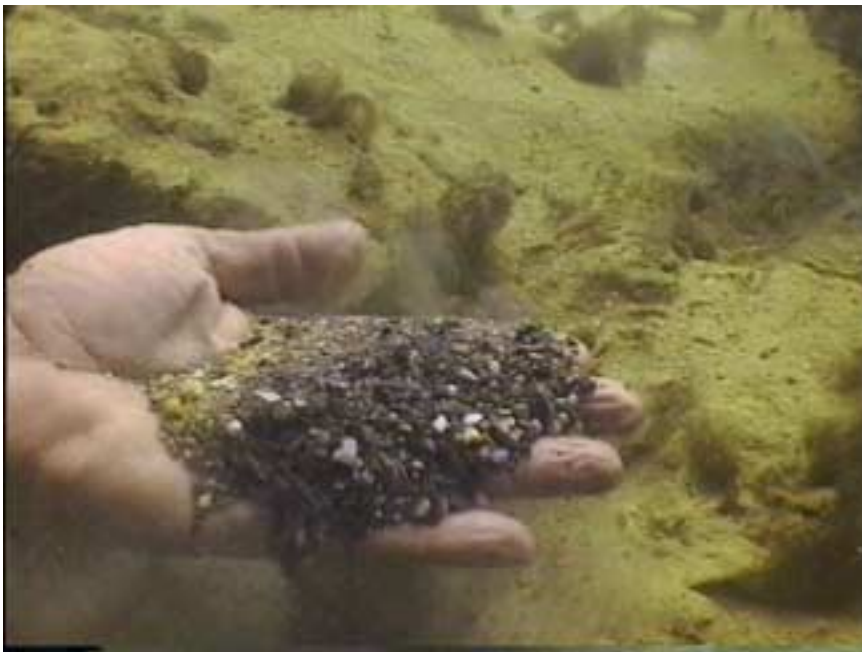
Photo WT9-11. Coral and steel debris pulverized by the demolition.
