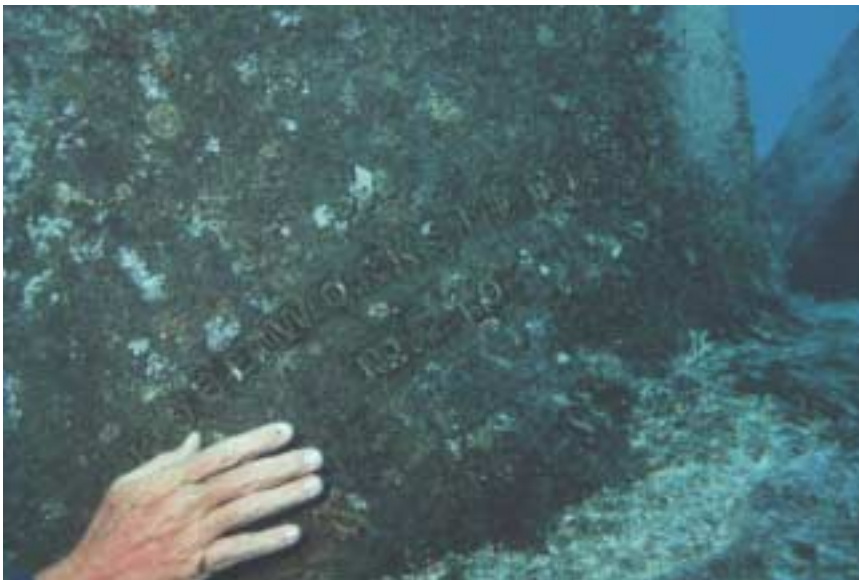
Photo WT13-12. Propeller manufacture cast into individual blades. This casting has Mitsubishi "3 Diamond" emblem and reads "KOBE WORKS MAY 1937, No. 210" Smaller ID reads "DIA 4.000m by PITCH 4.638m (not clear) ". Also on ID was numbers 12-3-22, indicated Japanese 12 th Year of Showa, meaning 1937, March 22 nd .
