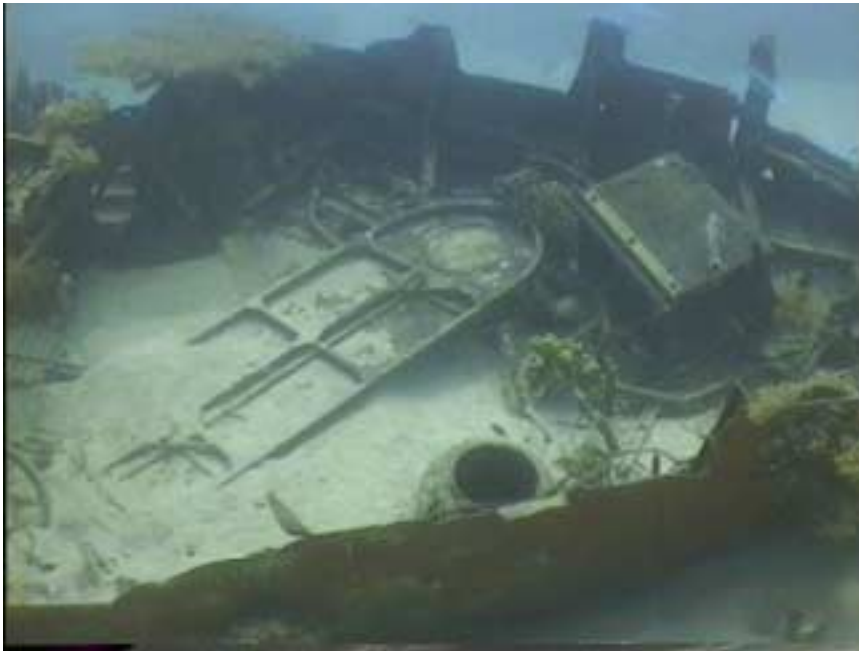
Photo WT5-4. Remains in the bow section of the flying-boat. Note the forward hatch door, a storage compartment box, and an engine cylinder in the photo.
