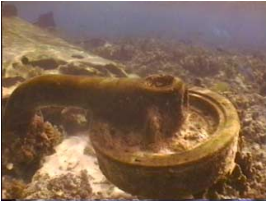
Photo WT1-7. Landing Gear Hub at the end of the severed right wing
