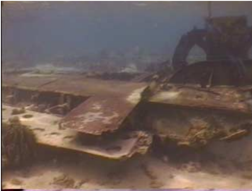
Photo WT1-9. Left wing section to the left of photo, with the remaining fuselage to the right. Note air brakes retracted in left wing assembly.
