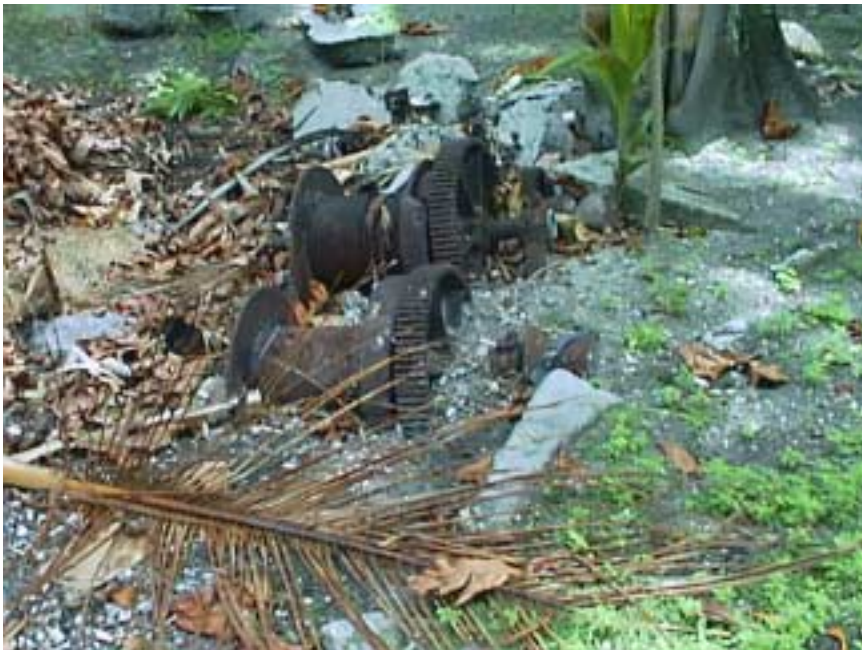
Photo WT6-7. A winch was set up inshore to haul boats ashore to the small dock.
