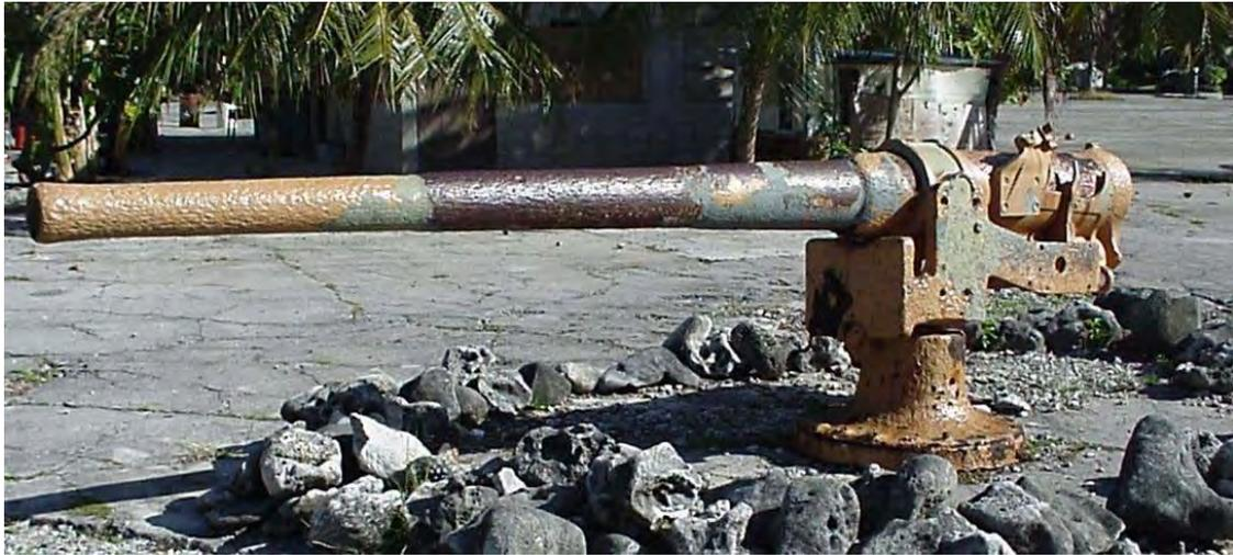
Photo 8 12cm Gun showing the zinc-rich and red-lead primer areas painted in 1992. The light green color at the opposite ends of the gun is the red-lead primer. The blue color in the middle is the zinc-rich primer.
