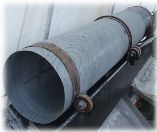
(Rotary screen with 3mm mesh)
