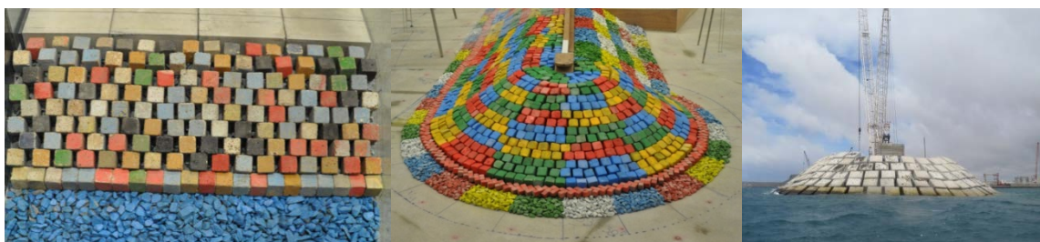
Figure 9.8 Stable, easy-to-construct solution with single layer cubes.
