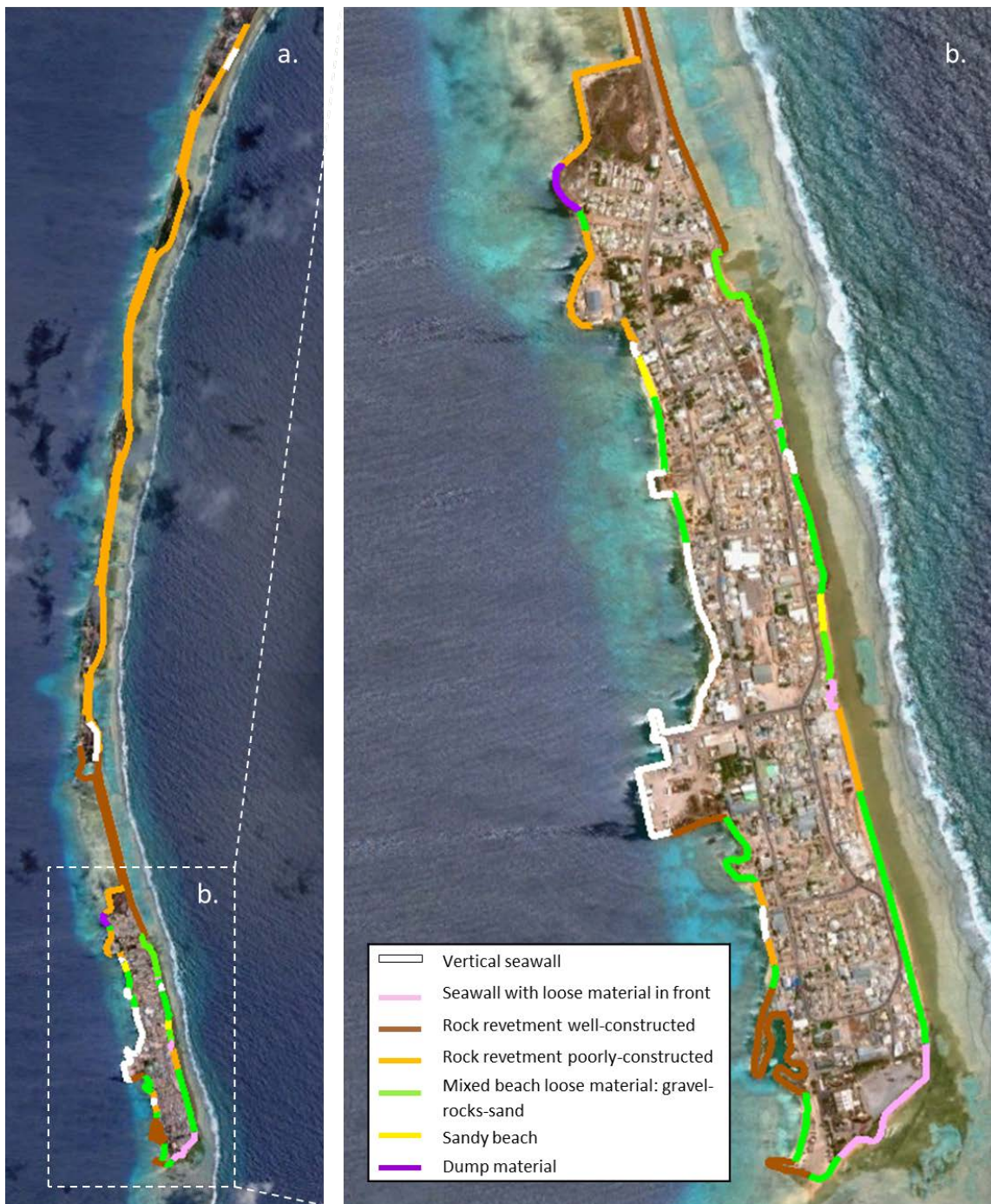
Figure 5.4 Observations of the types of coastal defences and/or materials, collected during the site visit.
