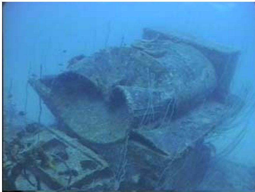
Photo MS3-8 Photo shows fuel tank section crushed by water pressure when sunk with the hatch and valves closed.
