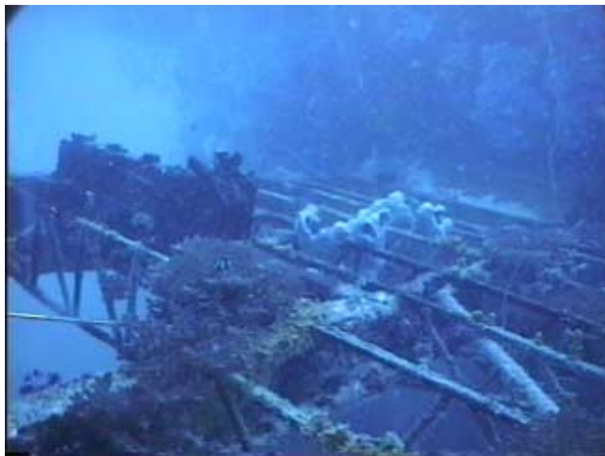
Photo MS10-6 Wing structure with aluminum framework.
