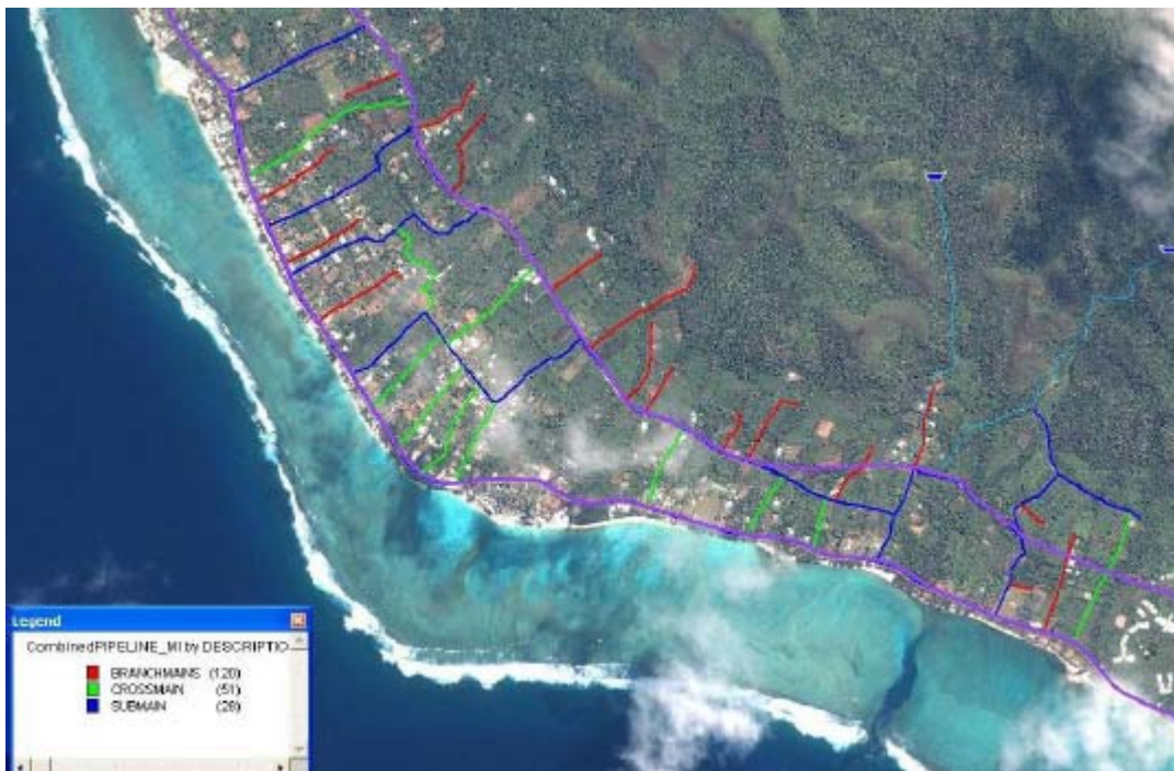
Figure 10: Enlarged view of the water reticulation system in south-west Rarotonga showing the branch-main (red), sub-main (blue), and cross-main (green) connections running from the ring main (purple).
