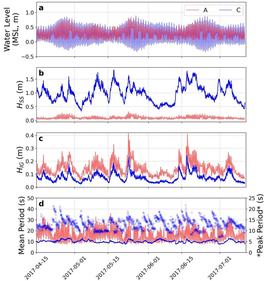
**Figure 2.** Observations from 2017 field deployment. Time series from sensor A (nearshore) and C (reef face) of: (a) 30-min average water level (MSL); (b) SS (0.04–0.3 Hz) significant wave height; (c) LF (0.001–0.04 Hz) significant wave height; (d) mean period (and peak period for sensor C only, shown in symbols).
