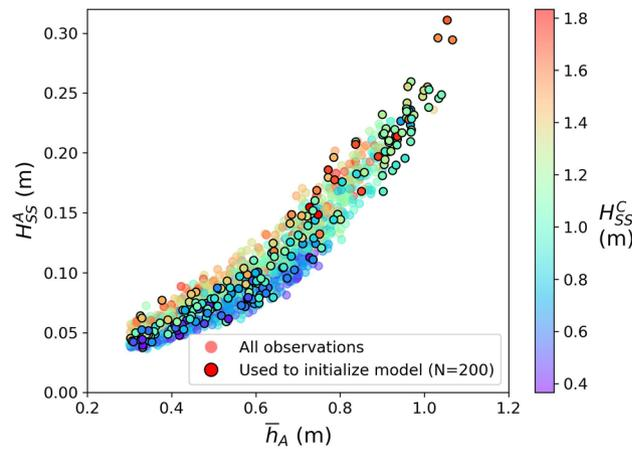
**Figure 3.** Nearshore (sensor A) sea-swell significant wave height as a function of mean water depth, colored by the observed significant wave height on the reef face (sensor C). All 30-min average observations with water depth > 0.3 m are shown; the 200 chosen for SWASH validation are marked with black borders. Nearshore sea-swell significant wave height is strongly depth-dependent, with weaker dependence on the reef face significant wave height.
