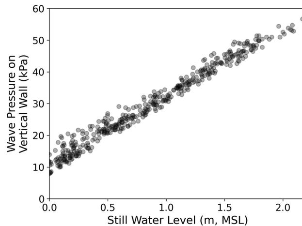
**Figure 9.** Modeled calculations of the maximum wave pressure on a hypothetical vertical breakwater constructed nearshore (sensor A), using the formulation from Goda (1974)<sup>40</sup>, as a function of still water level.
