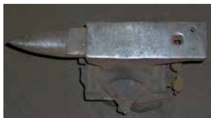
Figure 210: Top view of used London or English style anvil, by Fciron.
