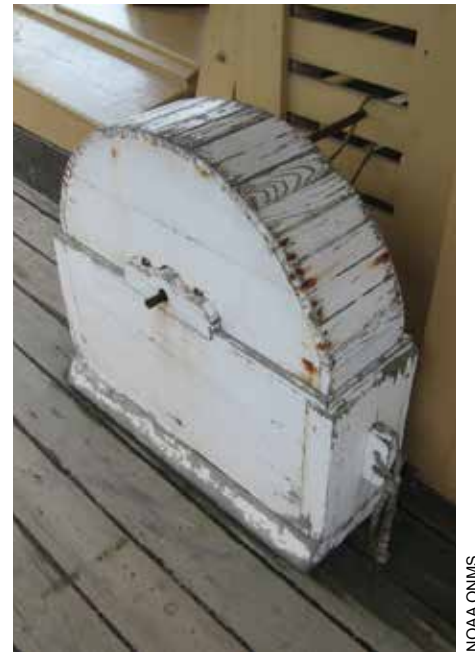
Figure 186: Wheel box with cover on board the whaler Charles Morgan , Mystic Seaport.
