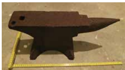
Figure 209: Anvil showing pritchel and hardie holes beneath the horn.
