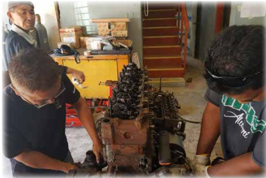
Japanese experts work with MIMRA mechanics to overhaul engines for the outer islands vessel Jebro.
