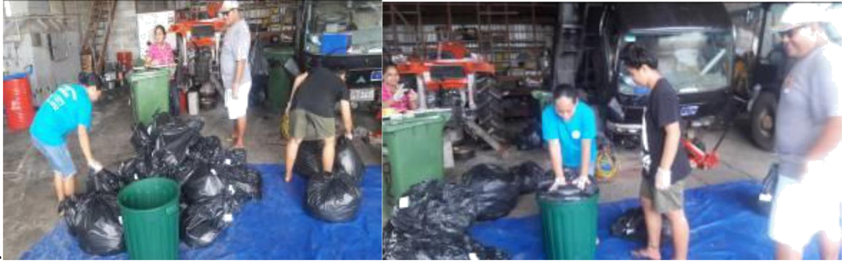
Measuring the Density of the Waste by Transferring all the Collected Waste into a Bin.
