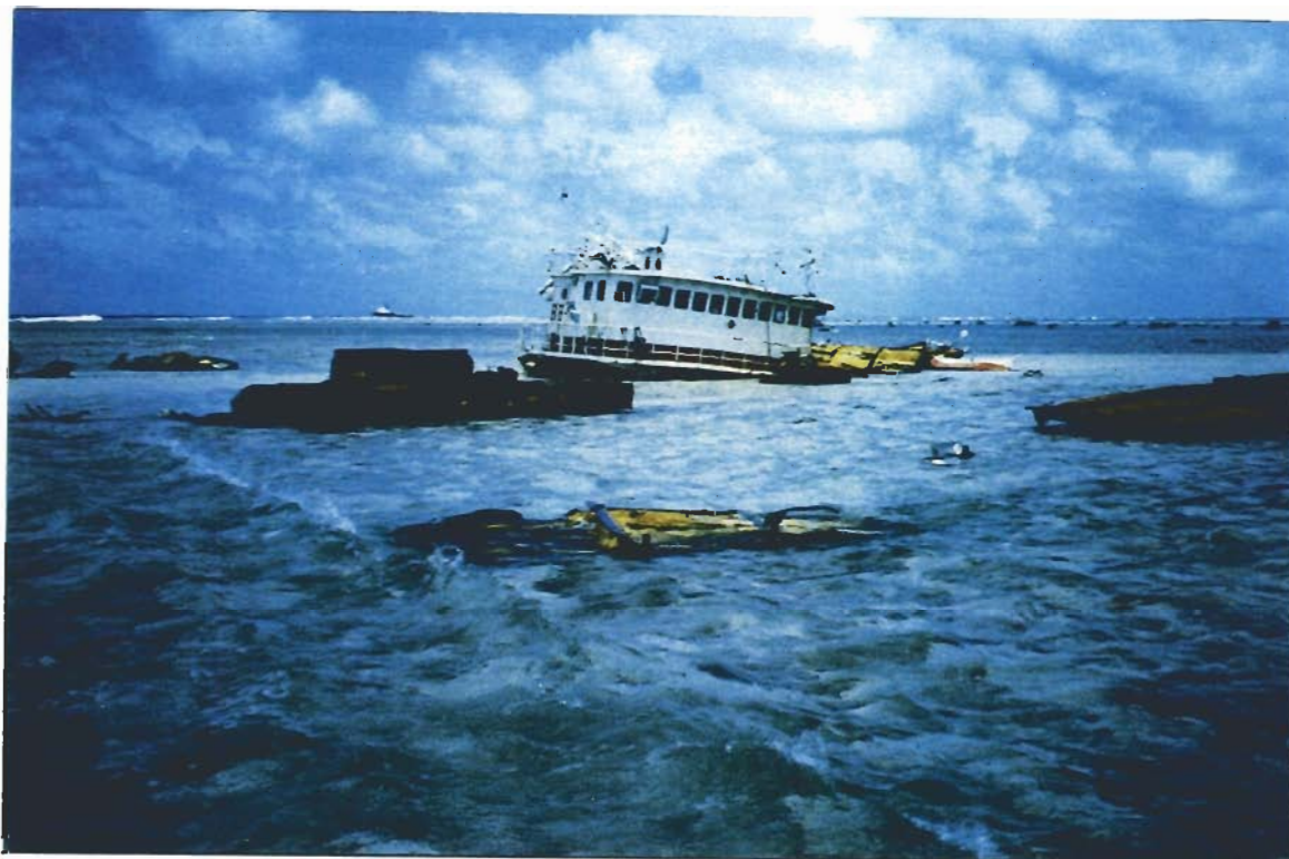
Figure 11 The bow section (top), wheelhouse and other pieces of wreckage (bottom) on the reef flat at Rose Atoll six weeks after the grounding.
