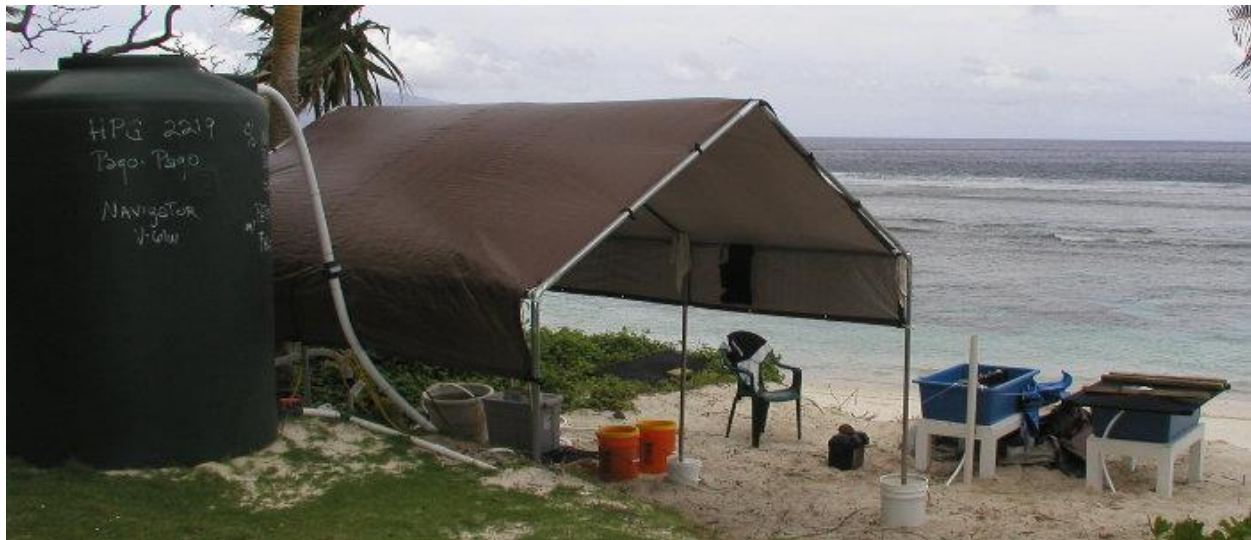
Fig. 6. The portable seawater system with a pump created by Lance Smith. A holding tank (left), shade or reducing intense sunlight, and experimental water tables (right).
