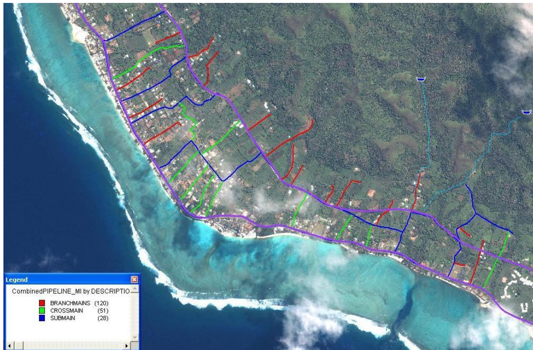
Figure 5: Enlarged view of the water reticulation system in south-west Rarotonga showing the branch-main (red), sub-main (blue), and cross-main (green) connections running from the ring main (purple).
