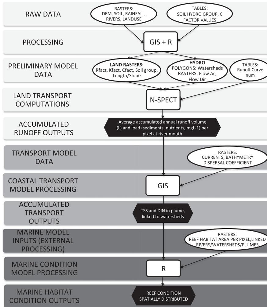
**Fig. 2.** Data flow diagram of the methods, and coupling processes, for the hydrological runoff (Step 1, light grey boxes), coastal sediment and nutrient dispersal and transport (Step 2, medium grey boxes), and marine ecosystem condition models (Steps 3–4, dark grey boxes).
