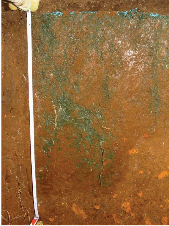
Figure 8.3. Visualisation of preferential flow paths by means of a brilliant blue dye tracer experiment using a disc permeameter.
