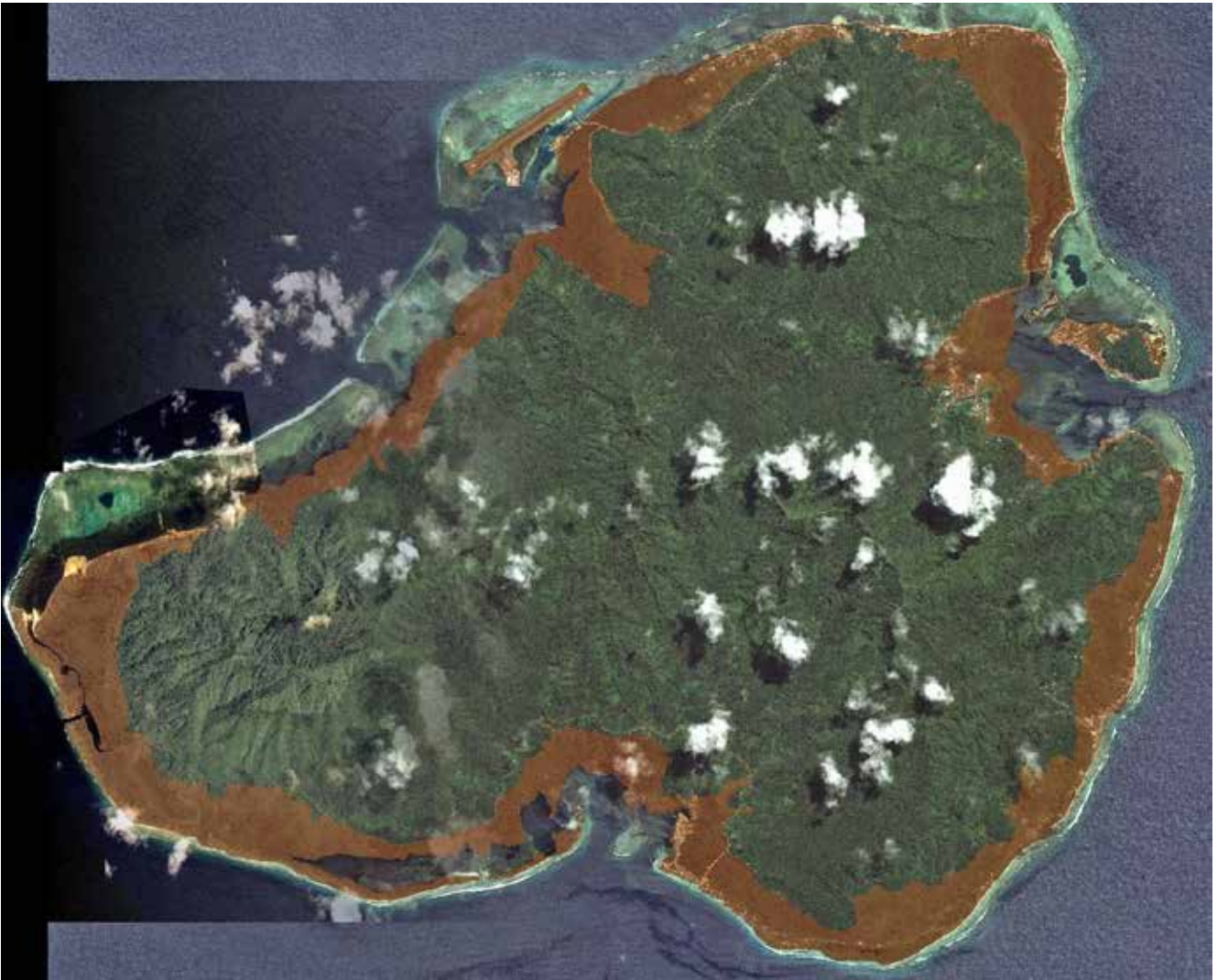
Figure 12: Low-lying coastal areas where restrictions on further development are required. The areas shown in red are largely below the 4 m MSL contour which is approximately 2 m above present day high spring tide level.
