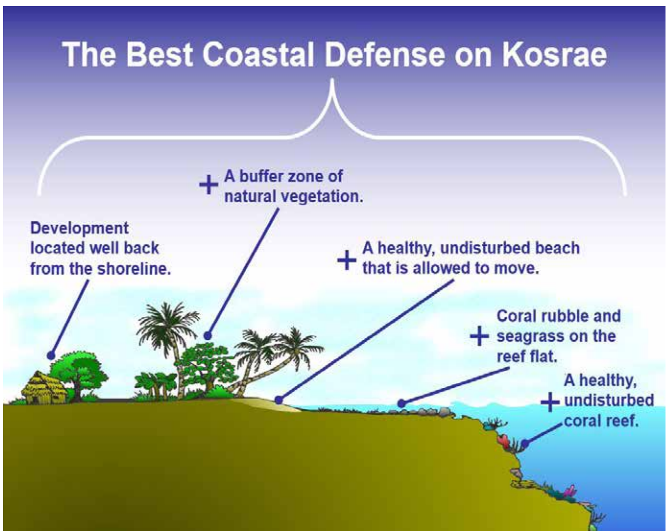
Figure 11: The best coastal defence on Kosrae. Awareness poster developed in 1999 by the Development Review Commission (now KIRMA).
