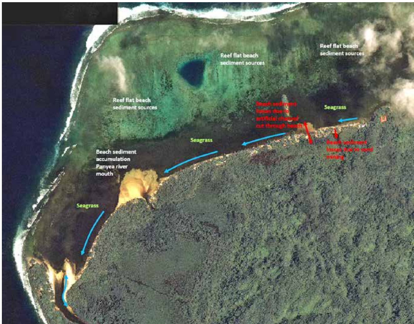
Figure B 4: Key sediment sources, longshore transport processes, and sediment losses along the Walung shoreline.
