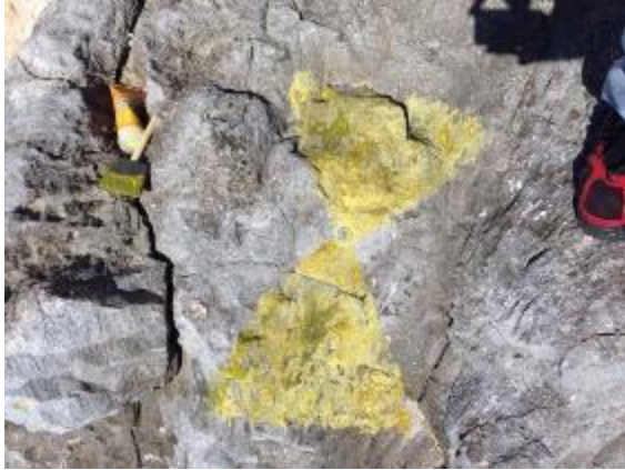
Figure 7: GCP 07 marker with yellow paint and view from aerial images
