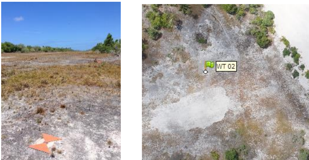
Figure 6: GCP 02 with orange tile and view from aerial photographs
