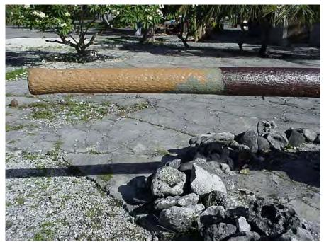
Photo 10 12cm Gun showing the red-lead primer area painted in 1992. The rust is where the zinc-rich primer was applied.
