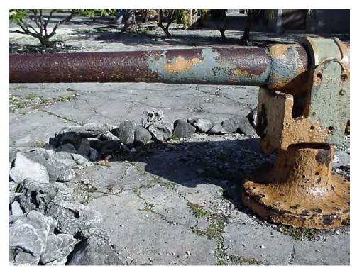
Photo 11 12cm Gun showing the zinc-rich primer area painted on the barrel in 1992.
