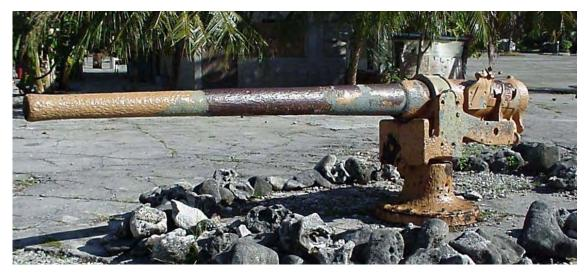
Photo 8 12cm Gun showing the zinc-rich and red-lead primer areas painted in 1992. The light green color at the opposite ends of the gun is the red-lead primer. The blue color in the middle is the zinc-rich primer.
