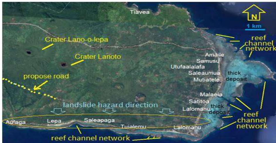
Figure 3 Coastal section between Aufaga of Lepa District to Lalomanu Aleipata Itupa I Luga as shown in the orange oval the most vulnerable area susceptible to generate landslide and rockfall during an earthquake. Blue arrows indicate the landslide direction and yellow lines shows reef channel associated with coastal erosion.
