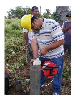
Water level measurement of monitoring bores
