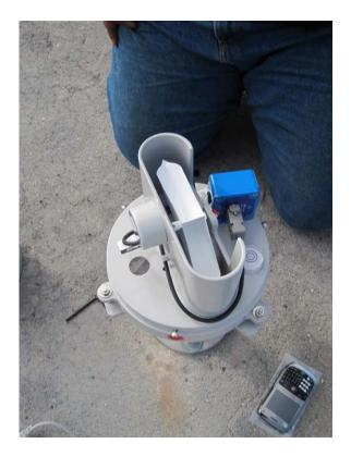
Figure 2: Gauge from above, without cover
