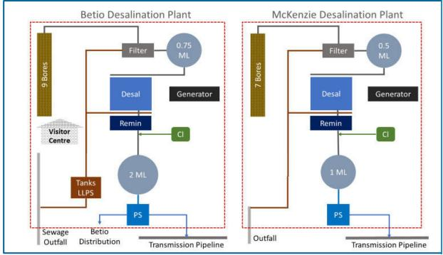
Desal= desalination, Remin = remineralisation, Cl = Chlorination, PS = permeate supply
