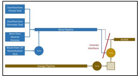
Figure 15 – Disposal of wastewater from the desalination plant in Betio
