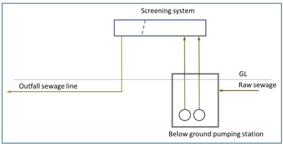
Figure 12 – Existing sewerage screening and outfall system
