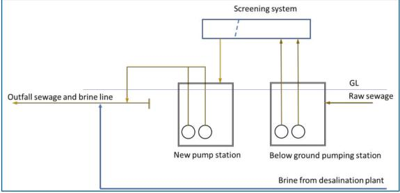
Figure 13 – New works required for sewage pumping station
