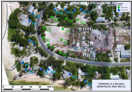
*Figure 20 - Desalination Plant Site at Betio Showing Bore Locations and Private Shallow Wells*
