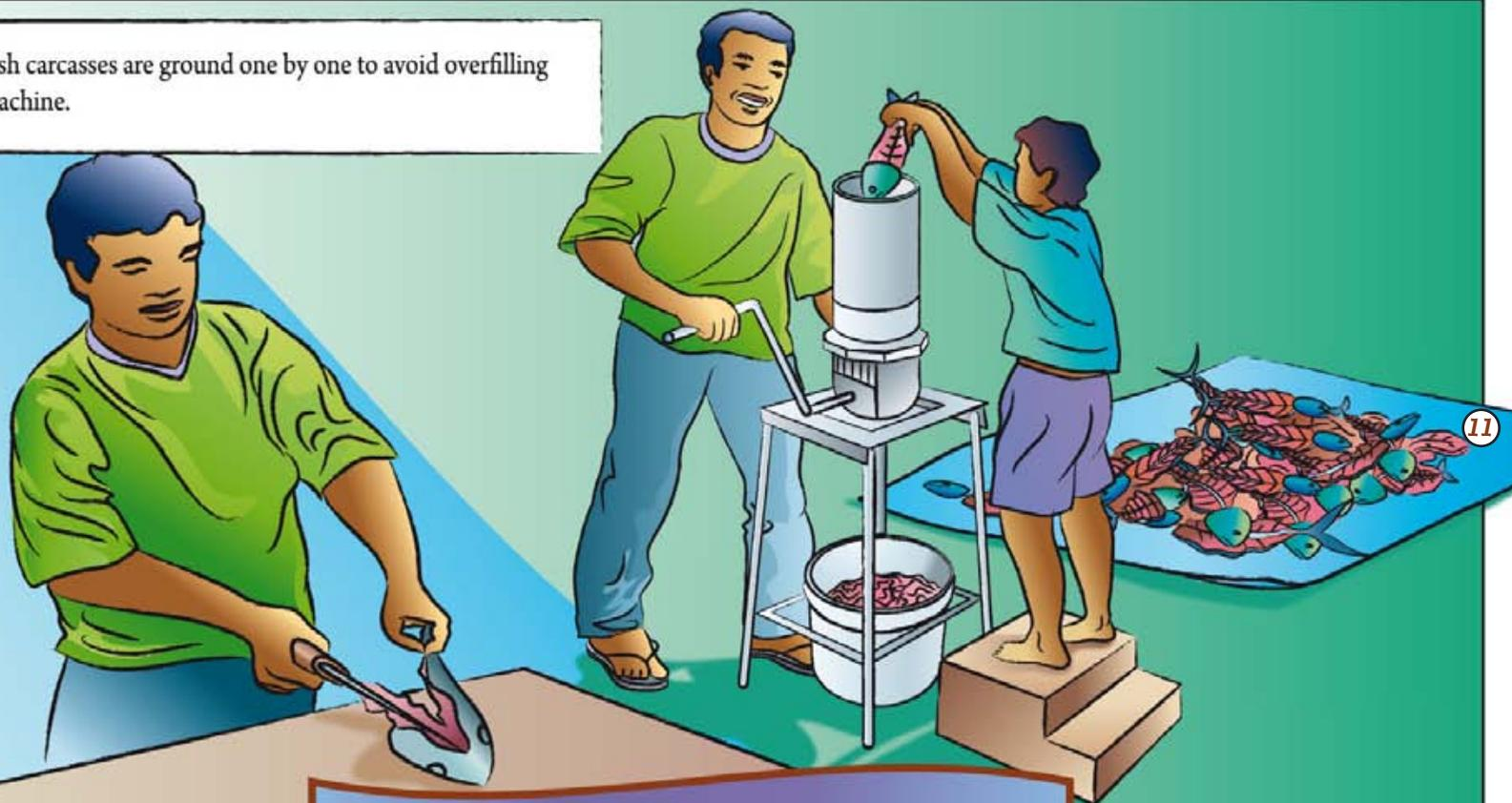
Large pieces of waste, like the heads of big fish, should first be chopped into smaller pieces to help the machine cope with them. You need to be very careful when doing this work!
