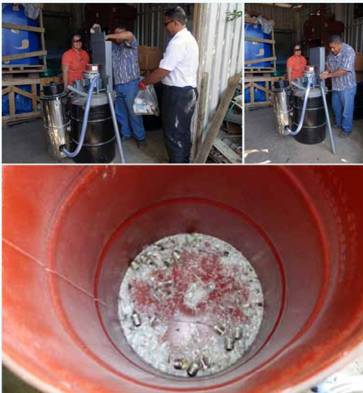
Figure 5.8. Operation of a bulb eater in Tonga
