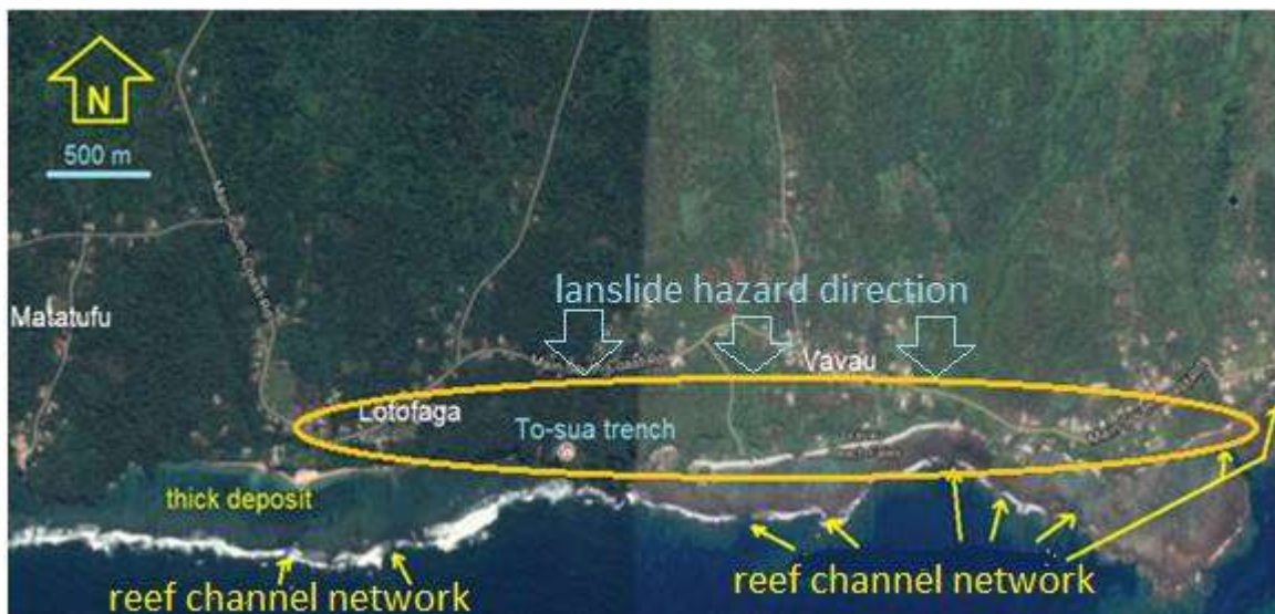
Figure 3 Coastal section between Matatufu and Vavau of the Lotofaga district. Orange oval indicates the high risk vulnerable area prone to collapse in the future. Blue arrows show landslide direction along this section. Yellow arrows indicate reef channels that contribute to major sand erosion in the coastal area.
