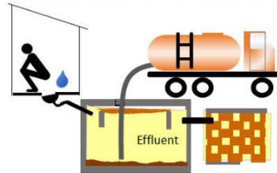
Figure 24: Emptying faecal effluent
