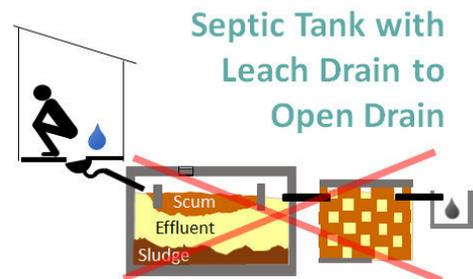
Figure 21: Septic tank with a leach drain discharging to the open drain
