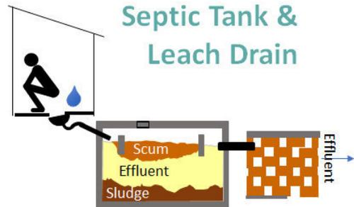
Figure 17: Sanitary Septic Tank Design
