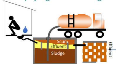
Figure 22: Faecal sludge emptying
