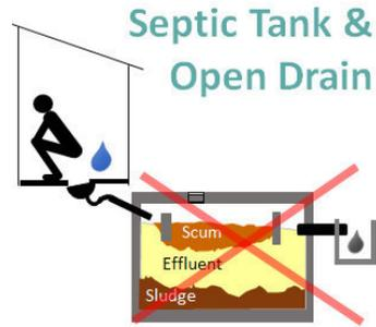
Figure 18: Unsanitary Septic Tank Design
