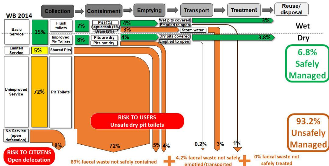
Figure 9: Shit Flow Diagram for Informal Settlements
