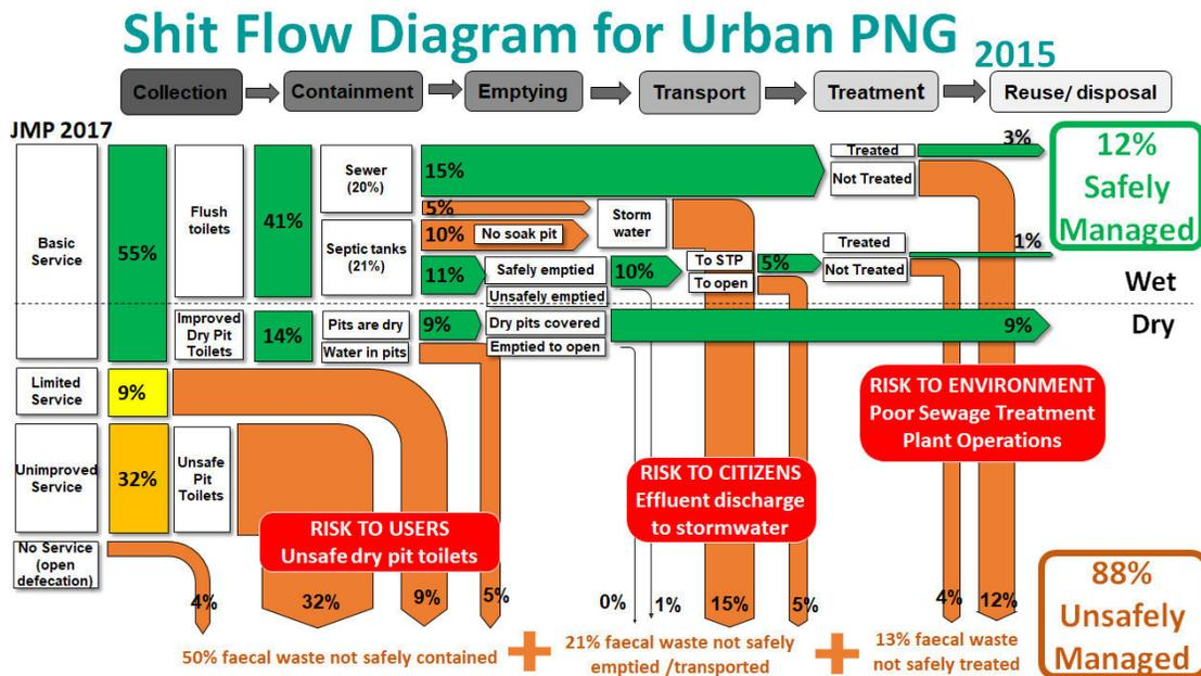
Figure 8: Shit Flow Diagram for Urban PNG (utilising 2015 JMP data)
