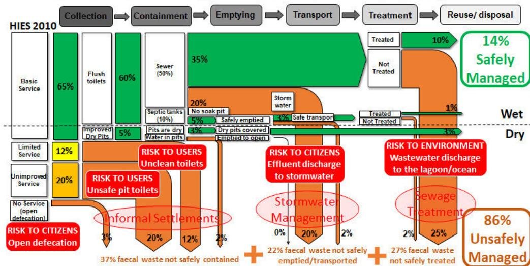
Figure 29: Shit Flow Diagram for Port Moresby (2010)
