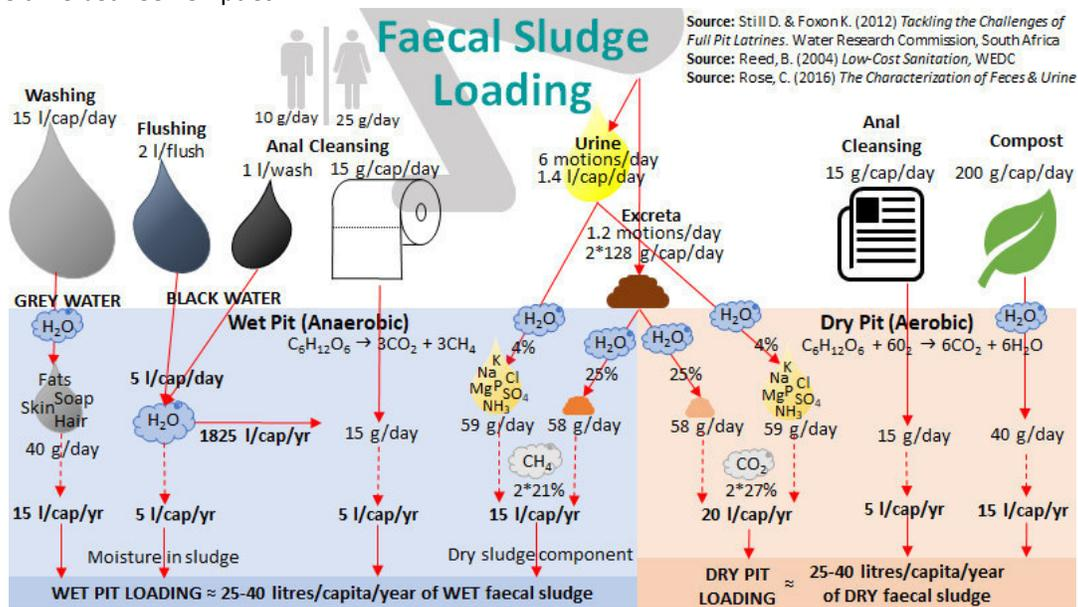
Figure 23: Faecal Sludge Loading Rates
