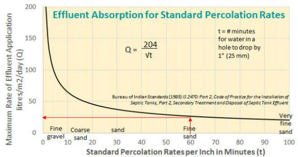
Figure 20: Effluent absorption for standard percolation rates
