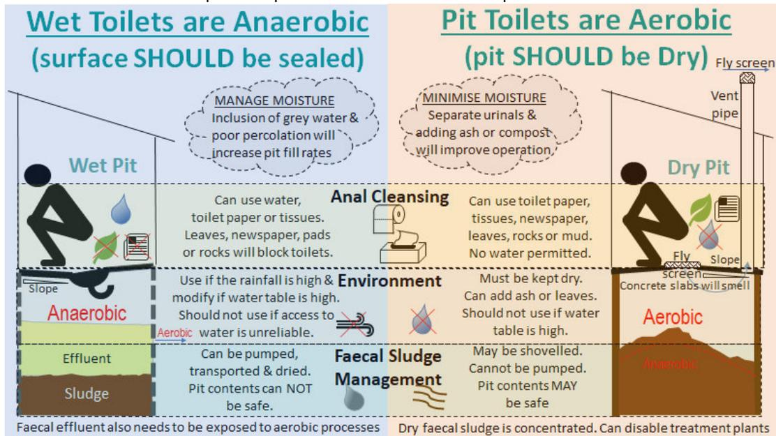
Figure 26: Aerobic versus anaerobic technology options
