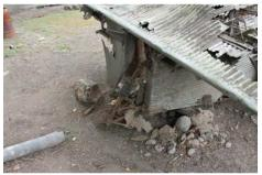
Figure 6 Object imbedded in soil will suffer higher corrosion that a object clear of the soil.
