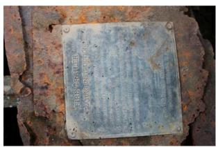
Figure 28 Typical advanced corrosion of parts in line with calculations. This piece is actively corroding as the "red rust" indicates.
