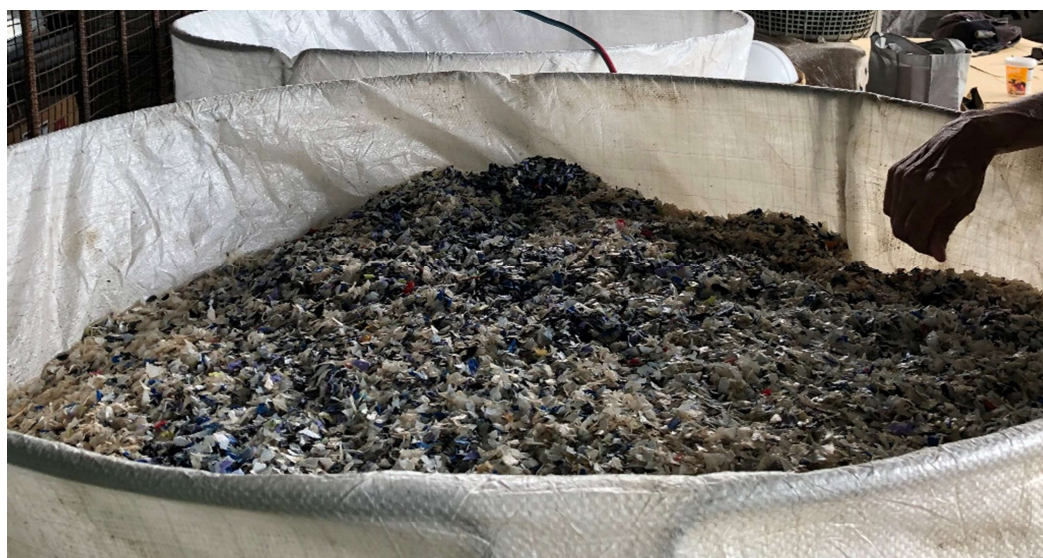
Figure 15: Shredded plastic ready for the pyrolysis machine at National Redemption Center, Palau. (Source: APWC, 2019)
