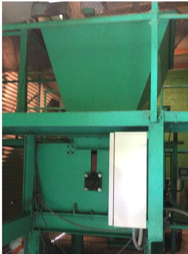
Figure 6: Counting machine at the National Redemption cent, Palau. It counts cans, glass bottles and plastic bottles. (Source: APWC, 2019)
