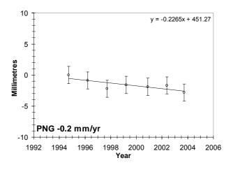
Figure 19. Movement of the SEAFRAME Sensor relative to the Tide Gauge Bench Mark.
