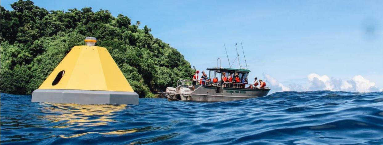
This buoy in Fagatele Bay continuously monitors ocean acidification and water quality parameters. Photo: Nerelle Que Moffitt/NOAA
