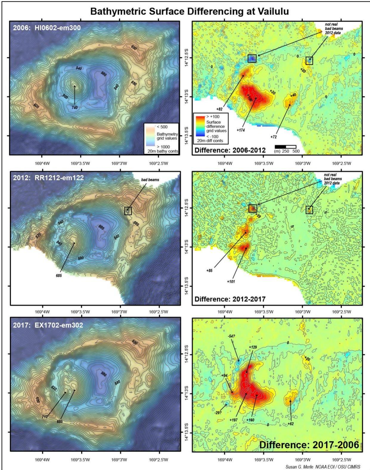
**Figure S.H.6.6.** Multibeam bathymetry of the crater at Vailulu'u Seamount (in meters), showing growth of the central cone over time. The map combines data from three different bathymetric surveys. Image: Susan Merle/Oregon State University and NOAA
