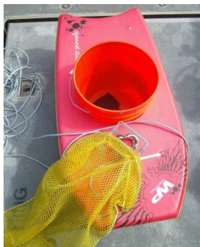
Figure 6.2.1. Flotation Device Used for Sampling.
