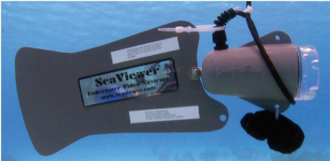
Figure 3 SEAVIEWER UNDERWATER VIDEO SYSTEM, OR DROP-CAM, USED TO RECORD BENTHIC COMPOSITION AROUND EACH ISLAND.
